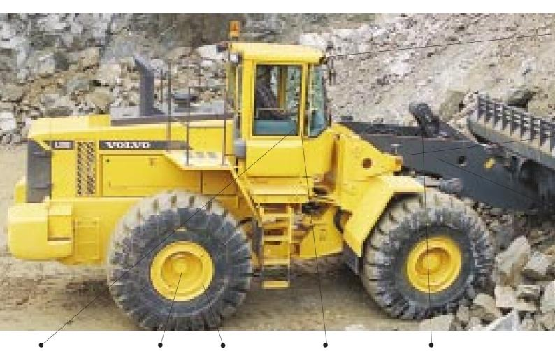
With Automatic Power Shift II, the operator can adjust the gear-shifting points according to the hardness of the work and save fuel. Fully-floating AWB axles for longer life.
