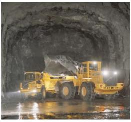
The Volvo L330D has Z-bar linkage and heavy-duty axles and frames that make it well-suited for tough rock handling. Limited-slip differentials, load-sensing hydraulics and the high-performance lowemission engine's high torque at low engine speeds give the loader the lowest fuel consumption in its class.
