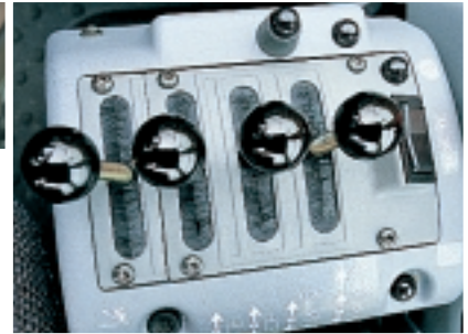
Pilot operated fingertip hydraulic levers provide easy control of the hydraulic functions. The adjustable hydraulic lever console also features a rocker switch for forward/reverse shifting and 1 st gear kickdown.
