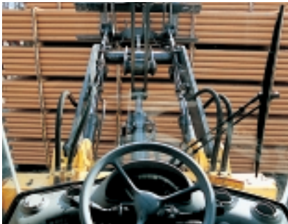
Visibility around the new attachment bracket and refined TP linkage make pallet forks even easier to use.
