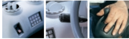
Left: Ten air outlets provide fresh filtered and climate-controlled air. Contronic II control panel allows direct access to all major monitoring functions.
