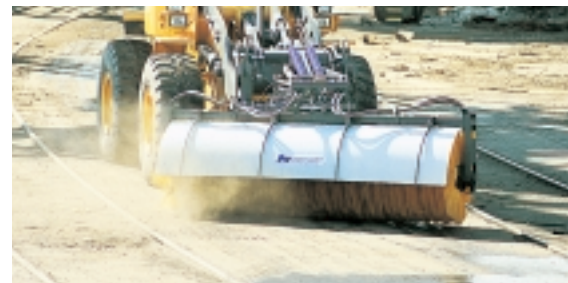
Thanks to the hydrostatic transmission, with its inching function**, the L50D can maximize power to the attachments while operating at very low speeds.
