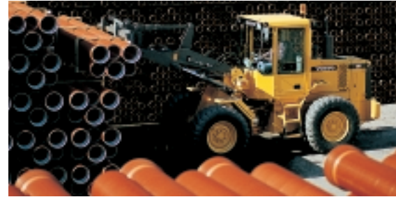
The TP linkage system facilitates long reach and parallel action even at the top.
