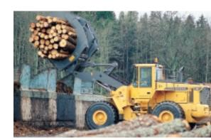
TP linkage comes into its own in timber applications. No other system provides such high breakout torque throughout the lift cycle.
