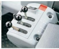
Pilot-operated fingertip hydraulic levers provide easy control of the hydraulic functions. The adjustable hydraulic lever console also features a rocker switch for foward/reverse shifting and a 1<sup>st</sup> gear kickdown button.
