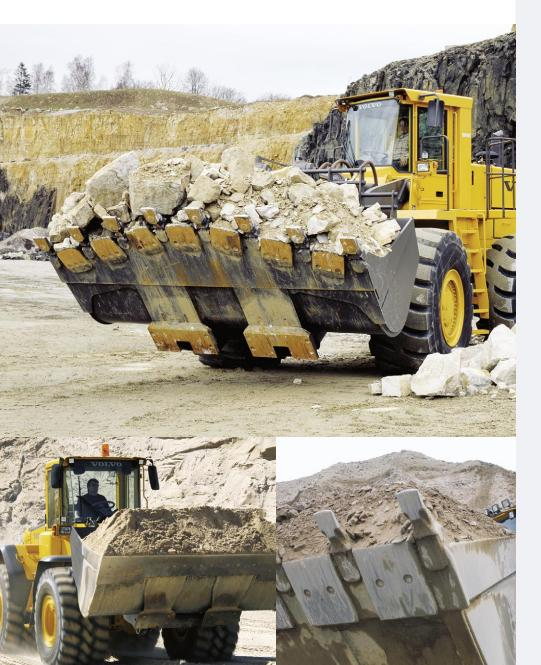
Side cutters with extra hardened and tempered steel wear plates provide high abrasion resistance (up to 500 Brinell)
