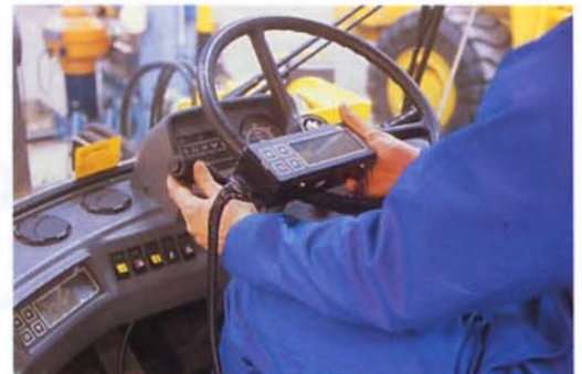
The Contronic system allows for quick service diagnosis. The system collects data from a number of analog sensors. Quicker troubleshooting gives shorter down time.
