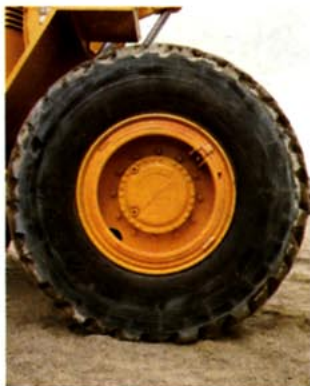
Big wheels provide stable operation, excellent negotiability and ample flotation in poor ground conditions.
