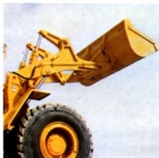
The rugged loader unit is made from materials of top quality. The sidearms have a broad attachment base on the anti-torsion frame.
