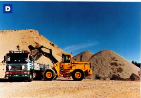
The TP Linkage maintains strength and parallel lift-arm action throughout the entire lifting range and provides the operator with excellent control of the load in all situations.
