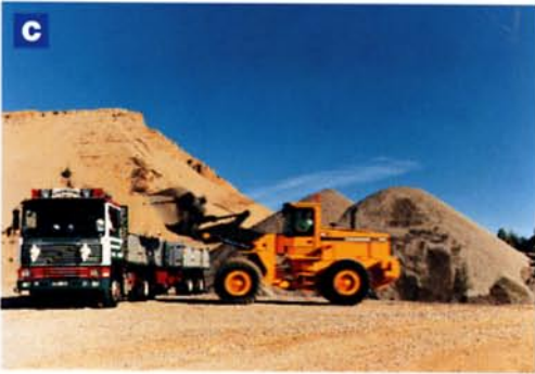
APSII, with program selector, ensures that the machine always operates in the correct gear. The operator quickly changes direction using the direction selector.
