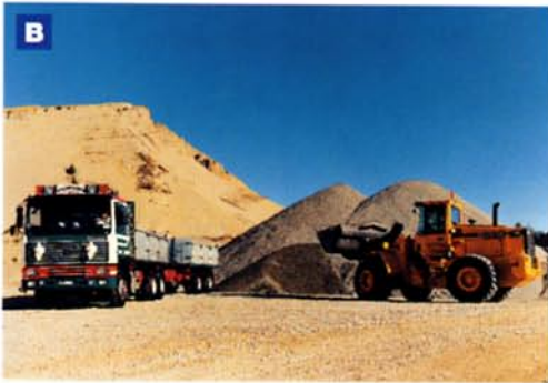
The load-sensing steering makes the wheel loader agile and provides smooth handling, irrespective of load. Compact lift-arm geometry and long wheelbase give excellent stability.
