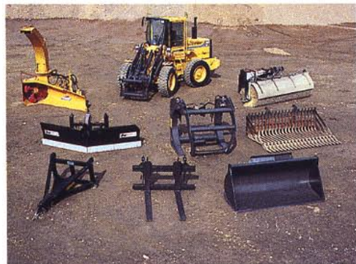
A large number of additional special-purpose attachments, produced in cooperation with a few selected Allied Suppliers, are available for Volvo BM wheel loaders. The photo shows snowblower, sweeper, folding plough and stone fork together with a selection of original attachments.
