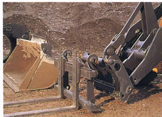
Thanks to the hydraulic attachment bracket, you can mount Volvo BM genuine attachments in a few seconds.
