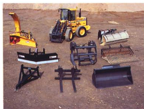
A large number of additional special-purpose attachments, produced in cooperation with a few selected Allied Suppliers, are available for Volvo BM wheel loaders. The photo shows snowblower, sweeper, folding plough and stone fork together with a selection of original attachments.
