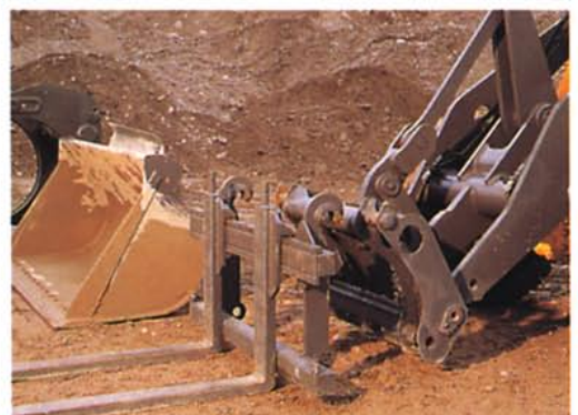
Thanks to the hydraulic attachment bracket, you can mount Volvo BM genuine attachments in a few seconds.
