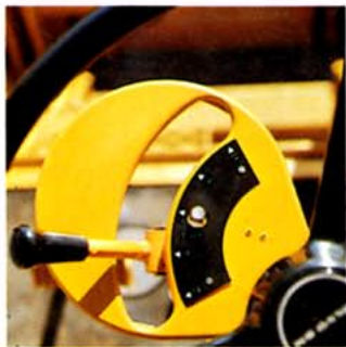
Easy to change gears with tight, precise positions. Safety start.
