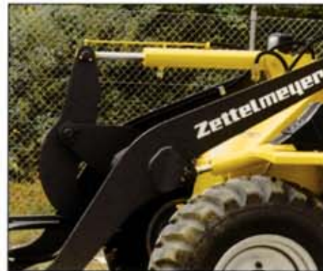
Z-bar loader-linkage - robust multi-purpose loader-linkage with high breakout and lift forces. Powerful in loading and production.
