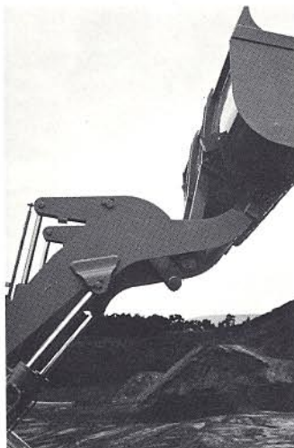
Z-kinematics for optimum breakout force.
