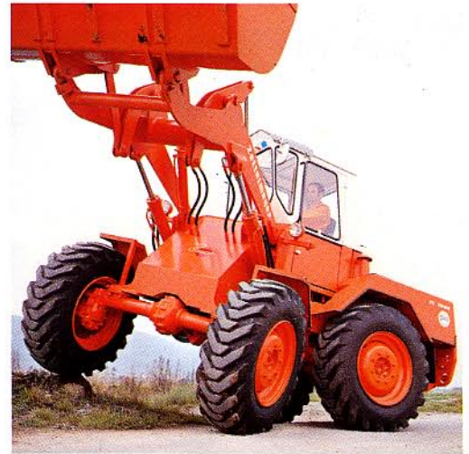
Exceptional cross-country mobility from oscillating articulated steering.
