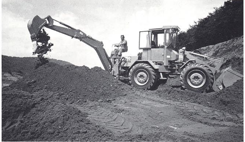
The standard rear mounting plate, here fitted with the high-performance ZL 22 C backhoe attachment HT 12. Digging depth 3600 mm (11'10"), discharge height 3200 mm (10'6"), 188° slew, max. side displacement 1260 mm (4'2"). Several other attachments are also available, please ask for details.
