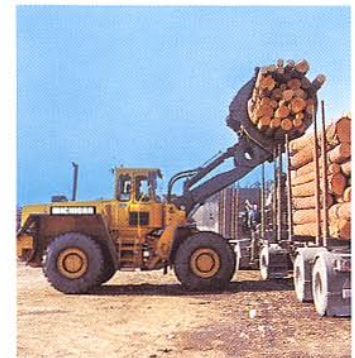
High tilt and rollback forces throughout the lift-arm movement permit effective, controlled unloading of timber from trucks.
