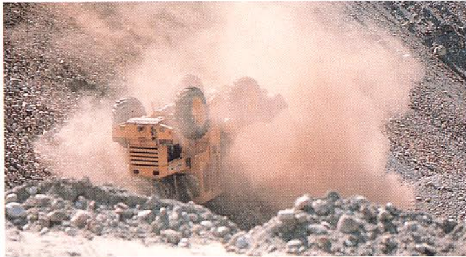
Michigan loaders roll over and over again down a rocky slope—and pass the test successfully.
