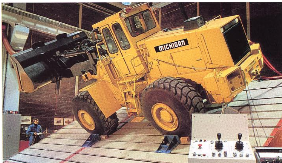
Sophisticated laboratory tests are combined with sustained field testing. In one test, machines have been forced to roll down slopes, with only superficial damage resulting. These tests complement the approved ROPS and FOPS tests.
