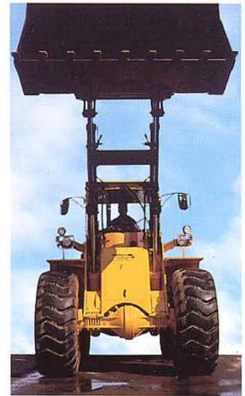
The symmetrical attachment of the cylinders gives very good reliability and extra good visibility through the loading unit.
