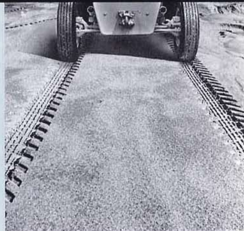
● Track width is identical for steering and driving wheels, improving performance on loose surfaces.
