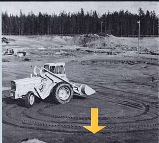
● Turning circle radius is only 5 metres (16 ft.), and can be even further reduced by using steering brakes.
