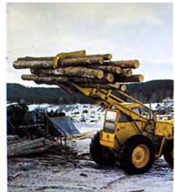
An LM 840 working at a tree processing station.
