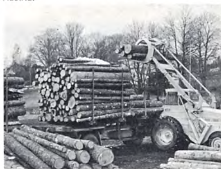
The generous lift height permits the full use of trucks fitted with high stakes.
