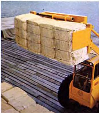
The hydraulic clamp simplifies the handling of pulp bales.
