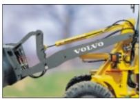
Parallel loader-linkage for good pallet work features - parallel lift of the working equipment for smooth loading and unloading in any lifting position.
