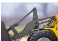
TP loader-linkage - combined loader linkage with tried-and-tested advantages: parallelity throughout the lifting range and controlled dumping even from the highest lifting positions.
