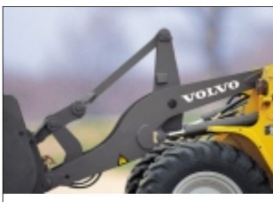
Z-bar loader-linkage - robust multi-purpose loader-linkage with high breakout and lift forces. Powerful in loading and production.
