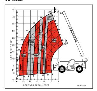
Always read and understand the published rated load capacity for the material handler model you are operating and do not exceed it. Load ratings per ASME B56.6 — 1992.
