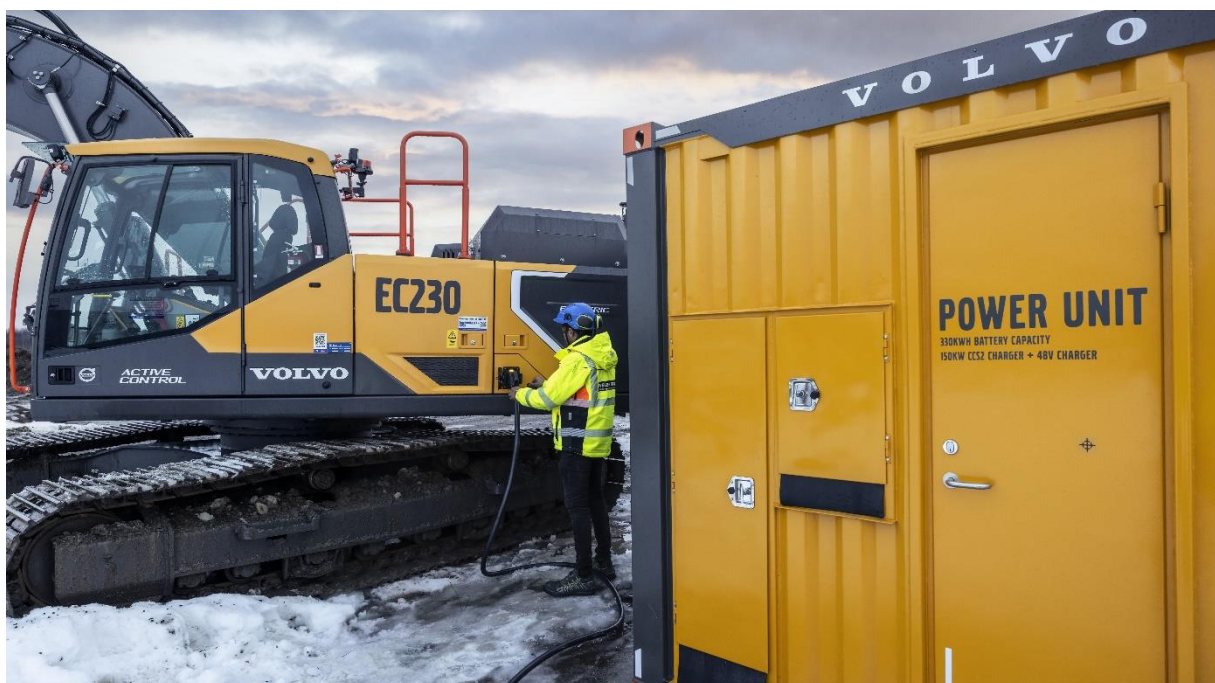
The mobile Power Unit supports charging in remote locations of larger machines like the EC230 Electric excavator.
