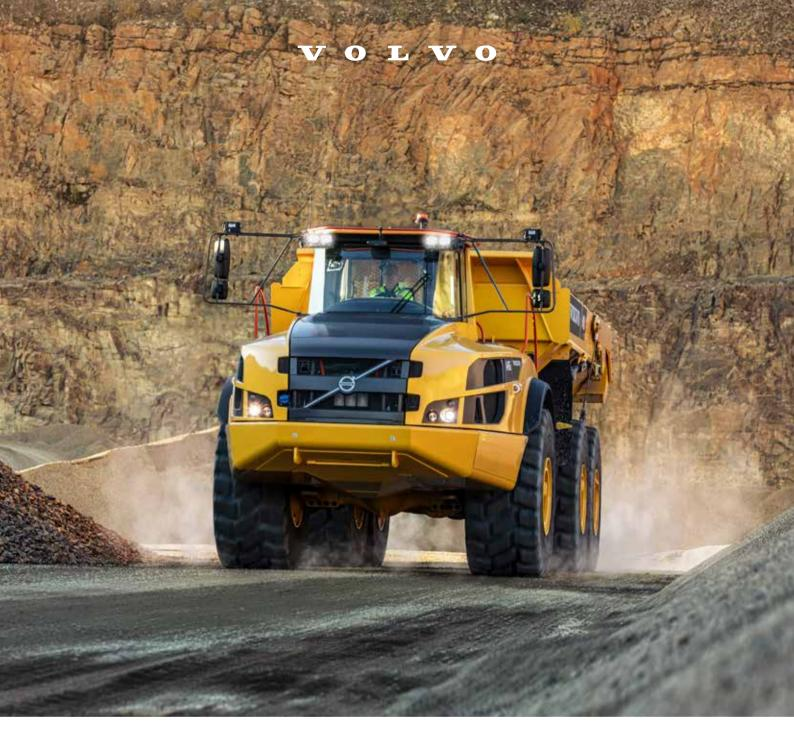
Volvo Articulated Haulers Imperial: 45.2 ton(us) / 90,389lb / 479HP Metric: 41t /41,000kg / 357kW
