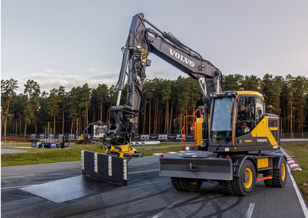
The recovery plate itself is insulated for the safest possible recovery of electric rallycross cars
