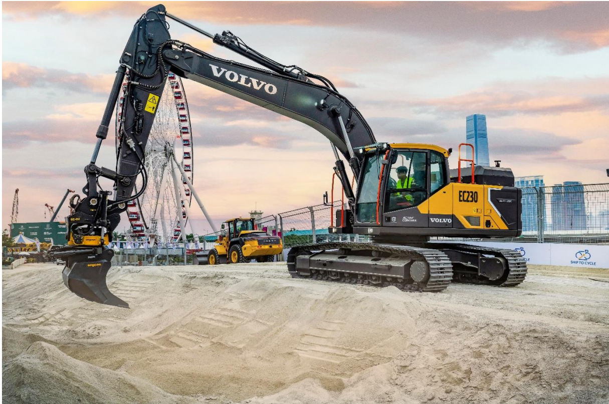
The EC230 Electric excavator offers zero emissions and precision excavation thanks to Dig Assist and the Engcon tiltrotator
